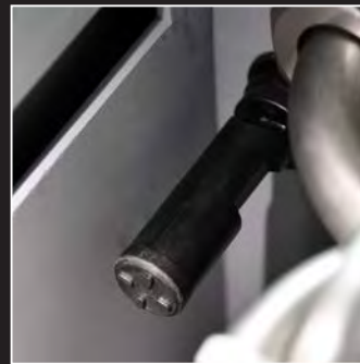
Level switch to control the water level in the boiler
