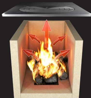
Phase 1: Accumulation and release of heat in the refractory combustion chamber during combustion.
